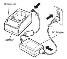
Insert the AC adapter's jack into the Charger and plug the power plug into a plug socket.
