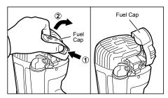
1) Press the Latch, then pull the Fuel Cap.
