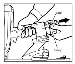
Firmly holding the grip, press the latches on both sides of the Battery to remove it.
