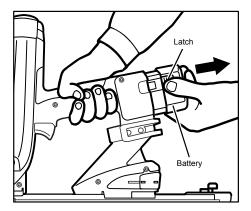
If the Battery is used up, remove it from the tool. Firmly holding the tool body, press the latches on both side of the Battery with your fingers to remove.
