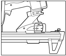
6 Make sure to align the Magazine with the Magazine Holder with no gap. Push the Remove Lever until it clicks.
