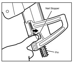
② Set the Magazine vertical and push the Nail Stopper to remove the Pin. Be sure that no pins remain in the Nose or Magazine.
