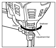
The driving depth adjustment is made by adjusting the Depth Adjustment Dial.
