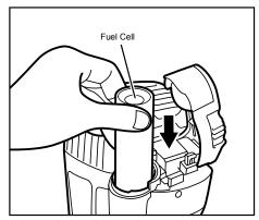
2 Insert the Fuel Cell into the tool.
