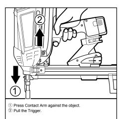
Firmly pressing the Contact Arm, pull the Trigger. The pins are driven into the object by combustion of the fuel.
