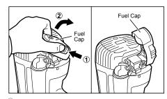
1 Press the Latch, then pull the Fuel Cap.
