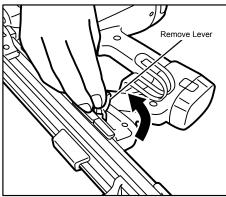
3 Pull up the Remove Lever and remove the Magazine from the tool.
